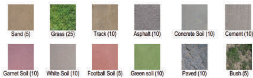
Fig. 3: Examples for targets ( 1 \times 1 \text{ m}^2 ) in the check areas and the number of reflectance values derived from spectrometer measurements per check area between brackets. As there are five measurements per target, the number of targets per check area is the number of measurements divided by five. For instance, there was one target over sand, but five targets over grass.
