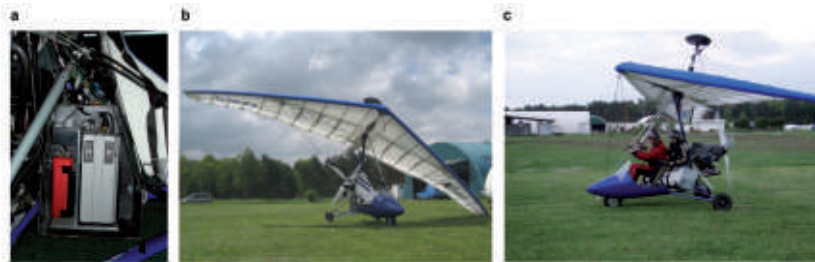
Fig. 4: a) AISA-EAGLE (400–970 nm) and GPS/INS-RT3100 mounted onto the microlight aircraft (Trike, D-MUFZ) of the UFZ, b) Microlight aircraft of the UFZ – D-MUFZ, c) Microlight aircraft for recording hyperspectral data – landscape level.
