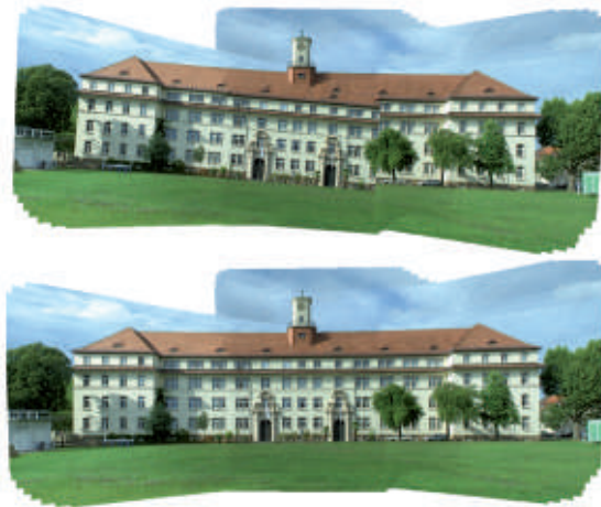
Fig. 2: Mosaicking of 355 video images of size 720 \times 576 pixel. Top: Image alignment by considering consecutive links only. Bottom: Result after the adjustment of two loops.
