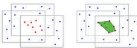
Fig. 3: Number of common points (red – left) and area (green – right) for overlap determination between three images.
