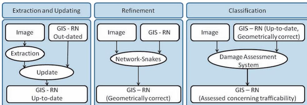
Fig. 2: The three moduls of the system (RN = road network).
