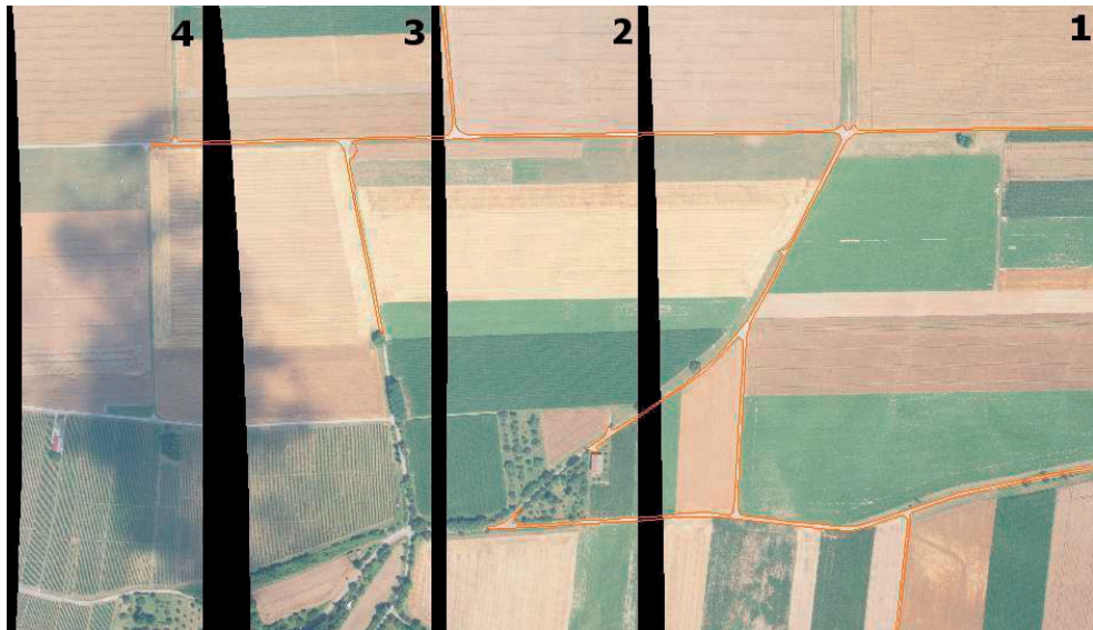
Fig. 10: Image sequence B: Result of road-tracking started from image 1 (red).
