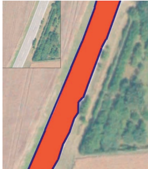
Fig. 1: Homogeneous road area (red) and border edges (blue), original image (top left).
