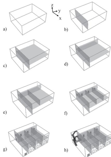
**Fig. 4:** Stepwise generation of a building with interior structures by applications of grammar rules. The stairs in h) can be obtained by additional grammar rules provided by SCHMITTWILKEN et al. (2007).
