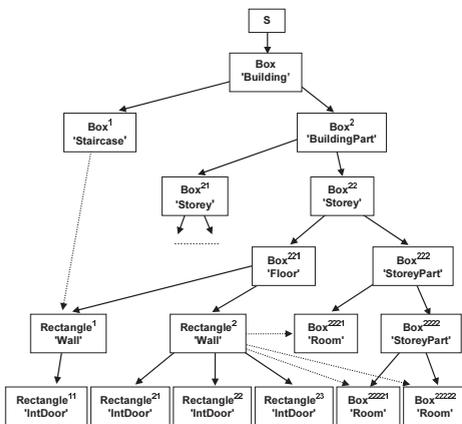
**Fig. 5:** Derivation tree for the generation of the building in Fig. 4. Bold arrows: rule applications; dotted arrows: relations derived from the constraints. The step of replacing a non terminal by a corresponding terminal is omitted.
