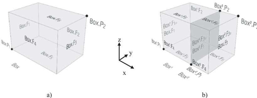
**Fig. 3:** Example for the application of rule R1. a) box before and b) after rule application with values *Direction* = ,x' and *Ratio* = 0,7. The rectangle shared by  $Box^1$  and  $Box^2$  is depicted in grey color.
