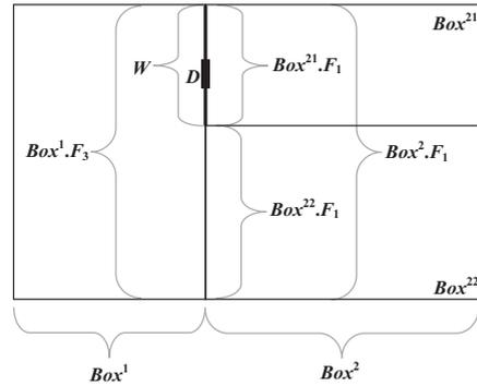
**Fig. 6:** Indoor scene where a door  $D$  is inserted in a wall  $W$  (view from above). From the constraints, it can be deduced that  $W$  and hence  $D$  are in the boundary of both  $Box^1$  and  $Box^{21}$ .
