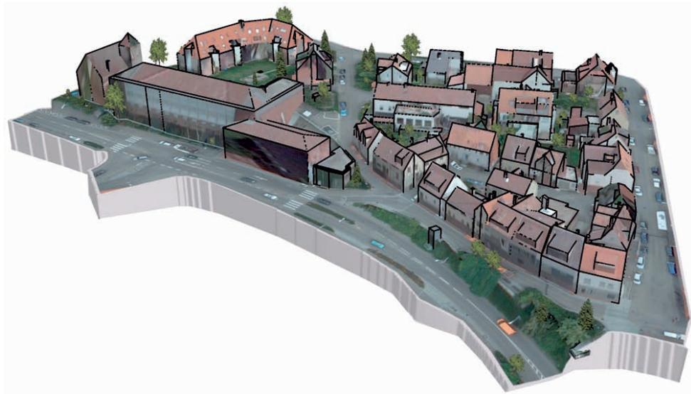
Fig. 1: 3D-aspect with stereoplotting results, Area 1 "Inner City", UltraCamX, 8 cm GSD.
