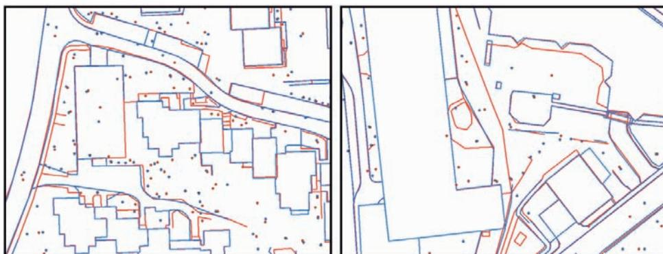
**Fig. 7:** Left: Area 2 "High Riser", comparison of stereoplotting results 8 cm GSD (red) to 20 cm GSD (blue), RMK. Right: Area 1 „Inner City“, comparison of stereoplotting results 8 cm GSD, UCX (red) to DMC (blue).
