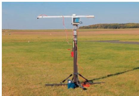
**Fig. 5:** BRDF-instrument GRADIS in operation.
