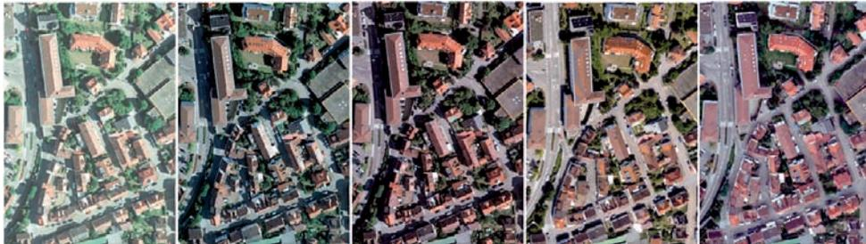
**Fig. 3:** Aerial images of Area 1 “Inner City” at individual flying times: from left to right: ‘08-07-24 RMK, ‘08-07-24 DMC, ‘08-08-06 DMC, ‘08-08-06 DigiCAM and ‘08-09-11 UltraCamX.
