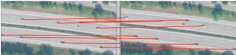
Fig. 6: Car tracking by normalized cross correlation of a group of cars detected in the first image of a sequence (left) to the second image (right).
