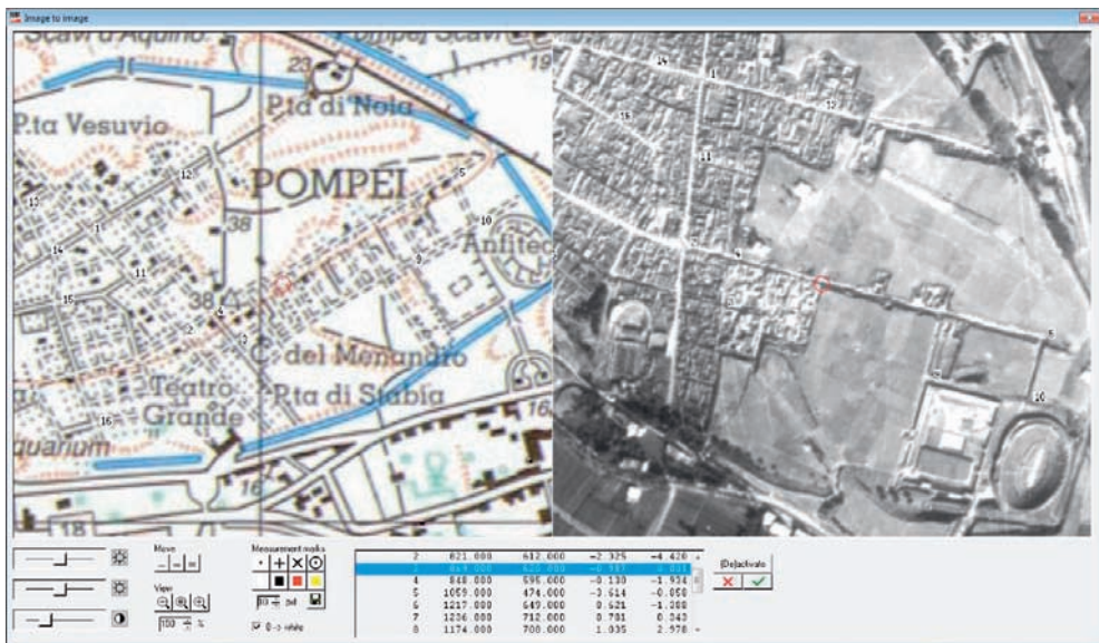
Fig. 2: Example of control points measured in both IGM map (left) and RAF aerial photograph (right) (screenshot from LISA software). Clearly to be seen is the different angle between the map and the photo and the distortion because of central perspective in the photograph before rectification.
