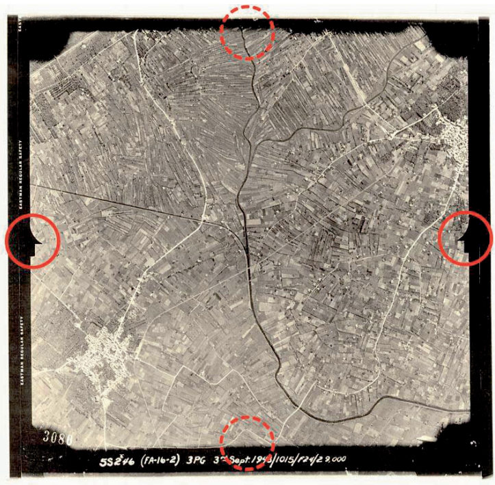
Fig. 1: Example of an RAF aerial photograph of 1943. Note that only two fiducial marks are visible on the left and right hand side.
