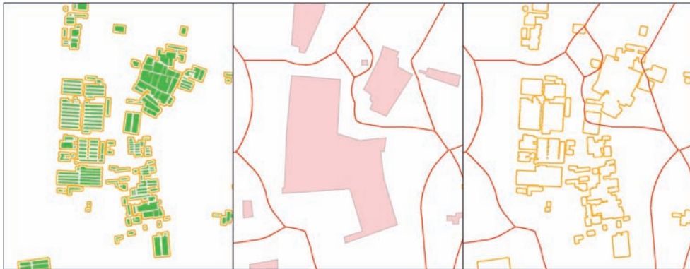
Fig. 6: Three-step-approach for establishing relationships between objects of data sets with dissimilar granularity; Creation of buffer polygons (bps) (orange) (left), Voronoi cells (Vcs) (red) of 1 : 50.000 (middle) and Result of overlay of bps and Vcs (right).
