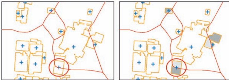
Fig. 7: Mapping results of the centroid point method (left) and the degree of the overlapping areas (right). The blue crosses are the centroids of the orange buffer polygons.
