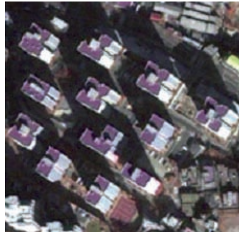
Fig. 4: Problem of shadow and inclination of buildings in very high and dense areas (Seoul, RGB: 3,2,1).
