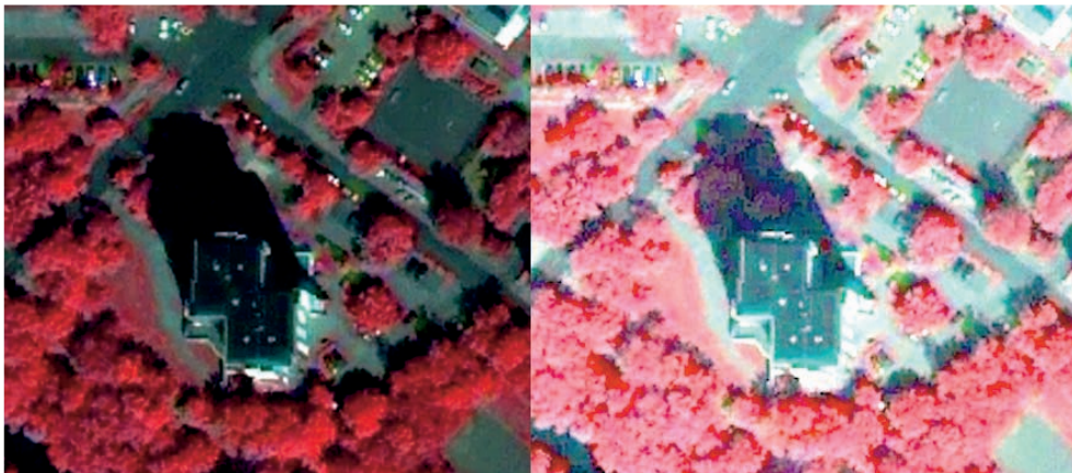
Fig. 3: Shadow-area after a histogram stretch, pan-sharpened image (Potsdam, RGB: 4,3,2).
