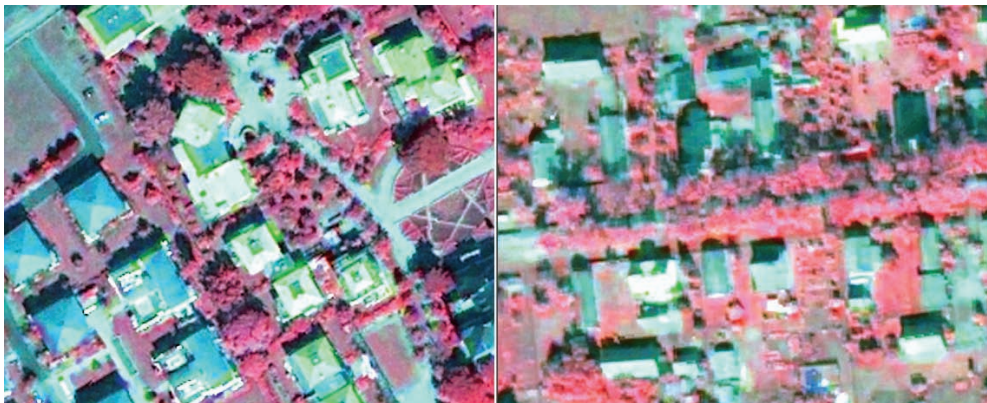
Fig. 1: Subset of a QuickBird-scene with 5,6° off-nadir view angle on the left (Potsdam) and 20,5° on the right (Lieberose), pan-sharpened image (RGB: 4,3,2).
