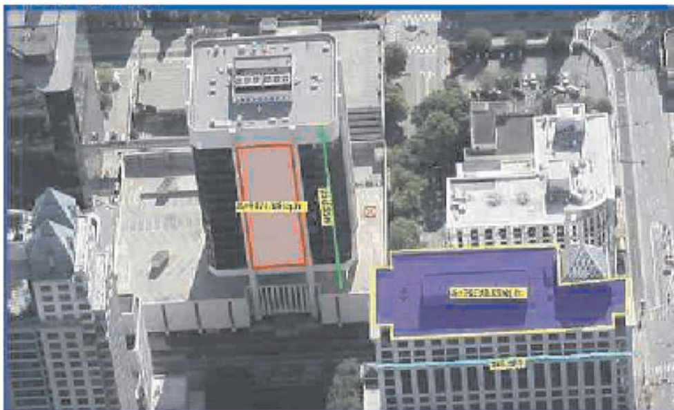
Fig. 5: 3D measurement in the Multivision oblique images.
