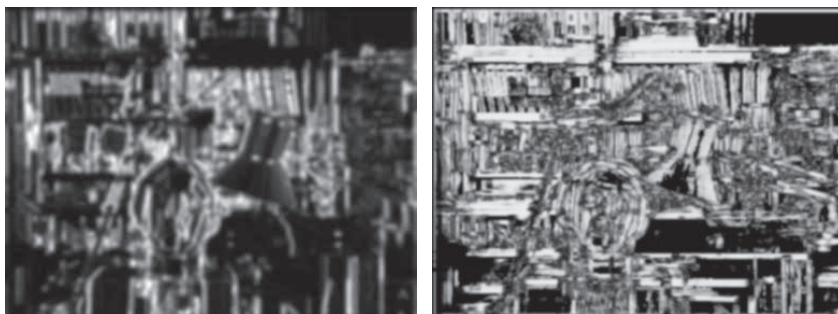
Fig. 7: Horizontal gradient (left); Maximum auto-correlation along the horizontal line ranging from outside the matching window to the search width (right).
