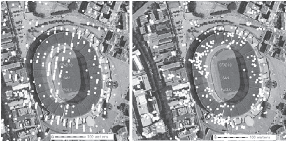
Fig. 4: Advanced geocoding of A-DInSAR results over the San Paolo Stadium of Naples (Italy). Pixel location without (left) and with (right) the correction based on the residual topographic error. An optical image of the area is on the background. This result was achieved by using an A-DInSAR technique described in LANARI et al., (2004), with 55 ERS images. (Images courtesy of Dr. RICCARDO LANARI from IRECE-CNR, Naples, Italy).
