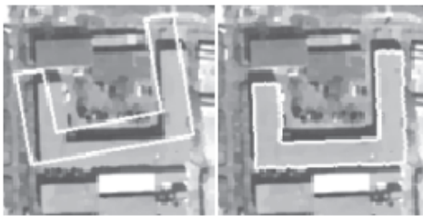
Fig. 6: Matching with DSM fusion ( \lambda_{flex} = cst , \lambda_{DSM} = 0.75 ). Left: initial state. Right: successful matching with DSM fusion.
