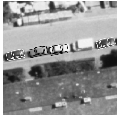
(d) Detected cars. White wireframe indicates car declared as "dark vehicle" and vice versa.
