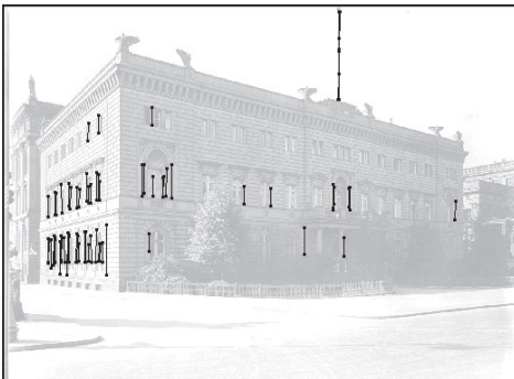
Fig. 5: Result of detection of three vanishing points.
